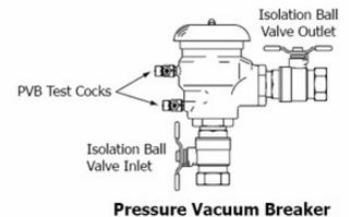
**Backflow Preventer Testing:** Pressure vacuum breakers and reduced pressure principle backflow preventers are required to be tested a minimum of once every three years but recommended yearly. The test must be completed by an ASSE certified backflow tester which most plumbing companies and several other companies in the water industry employ.
